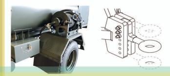
SCOPE: 600-gallon capacity mounted tank that is used for storing, transporting, and servicing aircraft with all types of ground support equipment fuels.
